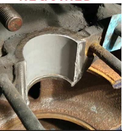
The damaged area was manually ground and cleaned prior to the application of the rebuilding material. Belzona 1121 (Super XL-Metal) was used as the rebuilding material. The product was mixed and applied over the damaged area and then the former was pressed against the product to achieve the desired dimensions. The former was removed after the product was fully cured.
